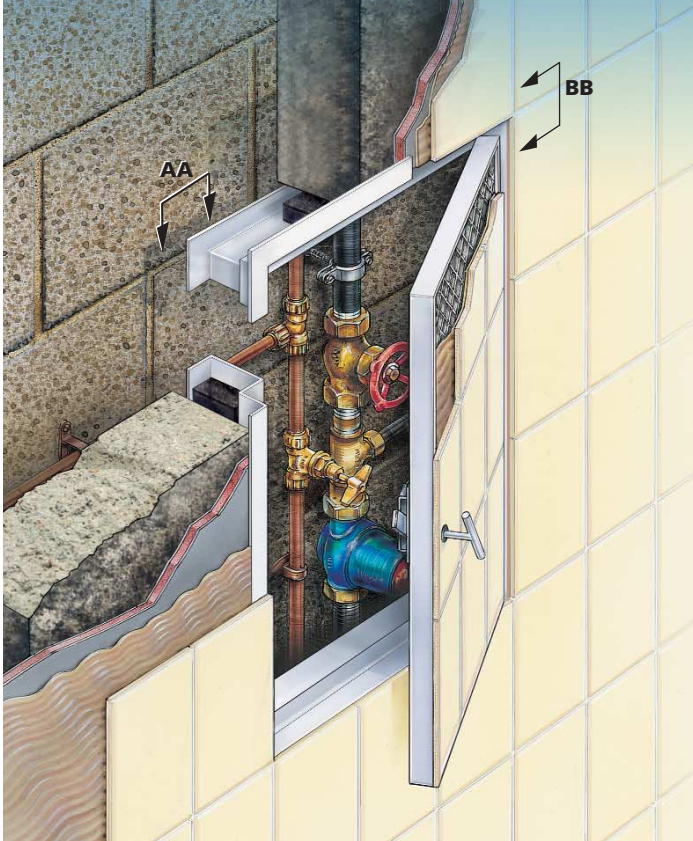
FIG 1 SECTION AA TILED WALL DOOR BUDGET LOCK OPERATED
